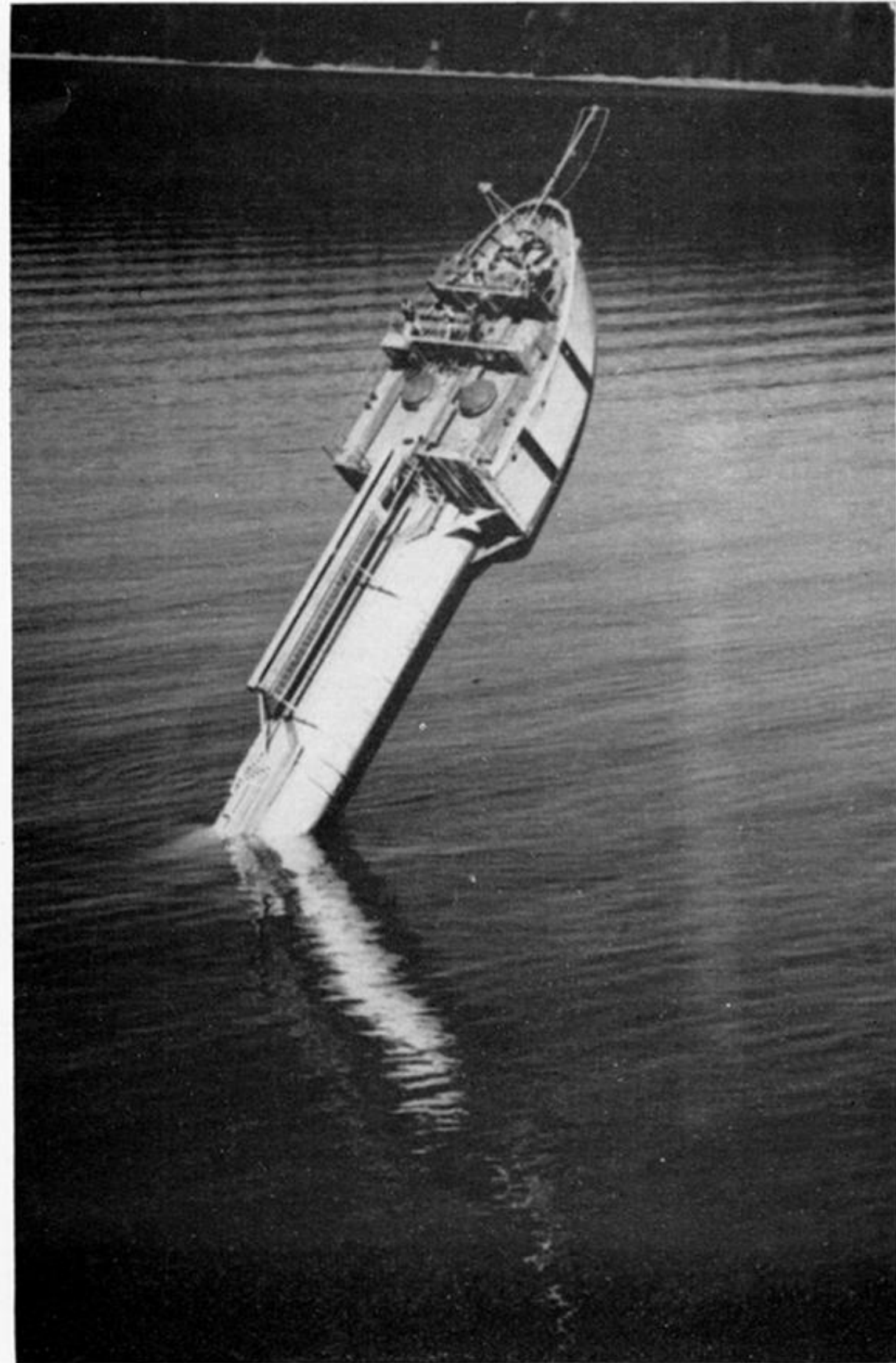
FIGURE 6. The vessel Flip in horizontal position, during flipping operation, and in vertical position (from Fisher & Spiess 1963).
